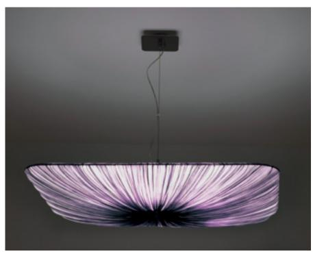
The Nara pendants are suspended from a brushed stainless steel ceiling plate 20 cm x 20 cm -8"x 8", by a 2 mm stainless steel cable, in adjustable heights up to 200 cm - 78" long, with a clear electrical cord. Shades can be balanced horizontally or up to 30 degrees diagonal.
